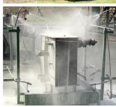
The I-CAT Fire Solutions' Localised Suppression System (LSS) was designed to protect your valuable production and industry equipment such as transformers, hydraulic power packs, conveyor belts (high risk areas like tail, head and tensioner pulleys) and fuel storage tanks against fire.
